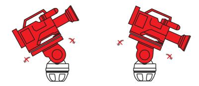
**3.** If the payload continues to move backwards when released, the balance is set too low. Raise the balance adjuster setting by one increment and retest.
