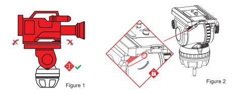
**(B)** If the payload tilts backwards, slide it towards the front of the fluid head. Re-lock the sliding balance plate.
