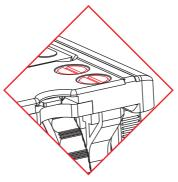
6. Mount the camera wedge plate and camera onto the sliding plate. It will lock automatically and the lever will click audibly back into its initial position.
