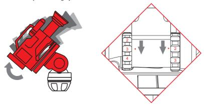
**5.** Tilt the payload through positive and negative angles of travel, checking that the payload remains at any angle of tilt unsupported.
