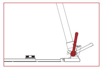
4. Unlock the three clamp knobs to allow the legs of spreader to extend as required.
