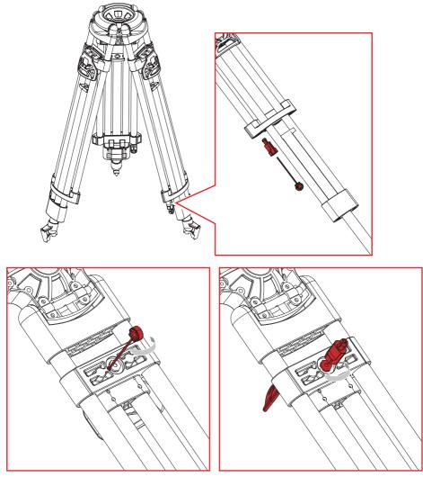
3. Keeping the quick release lever lifted. The lower adjustment screw is located as following. Using the given hex key, turn the lower adjustment screw clockwise to increase the brake force.
