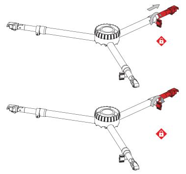
5. Secure tripod onto rubber feet by engaging three foot retaining straps to each foot of the tripod.
