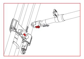
3. Release the buttons to lock the spreader in place.
