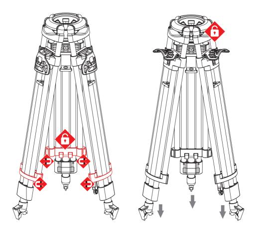
3. With the correct height achieved, lower the quick release levers to lock the legs in position.
